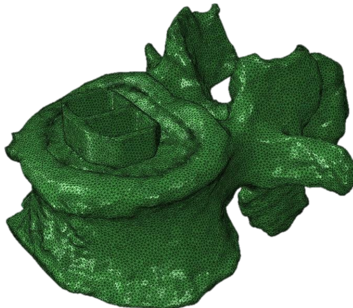
Figure 27: Representative image of the finite element model used in the study. The separately segmented endplate can be seen below the traditional geometry implant.
