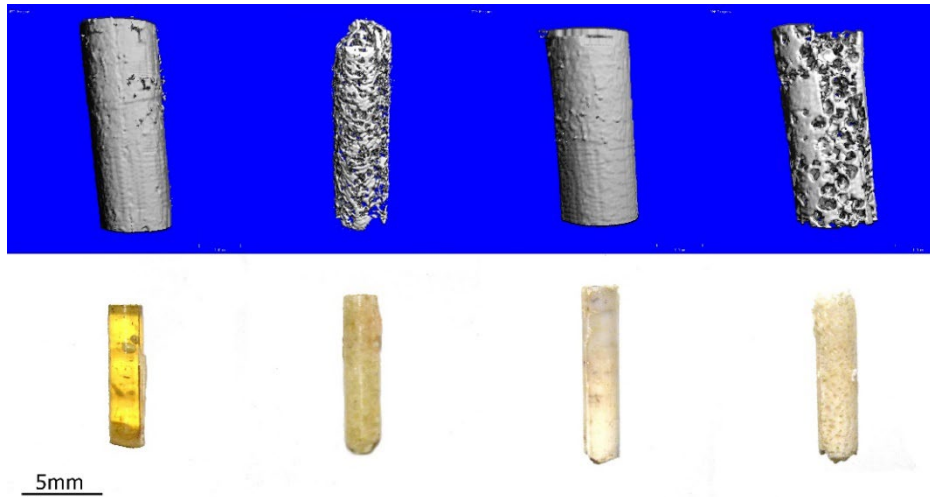
Figure 17: Representative images of implants. Micro-CT (top), Cylindrical implants for insertion in rat tibia (middle), and disk-shaped cylinders for cell culture (bottom)
